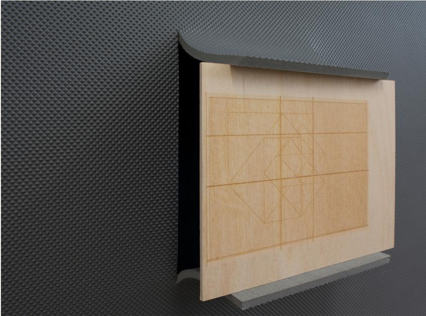
Laser on 3mm plywood clamped by shoe sole rubber
